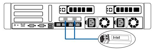
• On the NVR4X Premium 192/217 TB recorder, plug the Intel® SFP+ transceivers into the receptacles in the CNA card installed in PCI slot 2.
