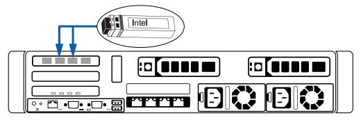
• On the NVR5 Premium 96/128/160 TB recorders, plug the Intel® SFP+ transceivers into the receptacles in the CNA/SAN card installed in PCI slot 4.
