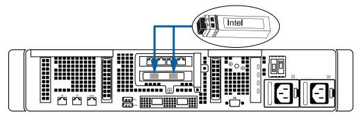
• On the NVR4 Standard, NVR4X Standard, and NVR4X Premium 64/96/128/157 TB recorders, plug the Intel® SFP+ transceivers into the receptacles in the CNA card installed in PCI slot 4.
