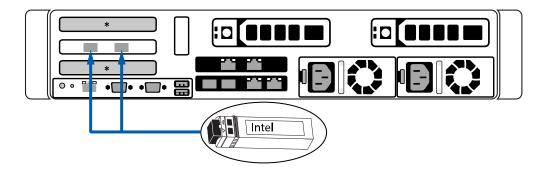
The NVR is now ready to be connected to the Avigilon Video Archive controller unit with the orange optical cables provided in the NVR Avigilon Video Archive Connectivity Kit.
