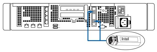
• On the NVR5 Premium 252/288/360/432 TB recorders, plug the Intel® SFP+ transceivers into the receptacles in the CNA/SAN card installed in PCI slot 1.
