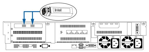
• On the NVR5 Premium 192/224 TB recorders, plug the Intel® SFP+ transceivers into the built-in 10G network card receptacles in PCI slot 1.
