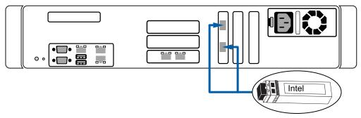
• On the NVR4 Premium recorder, plug the Intel® SFP+ transceivers into the receptacles in the CNA card installed in PCI slot 4.
