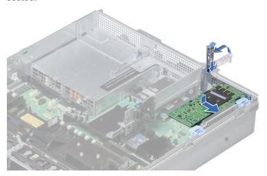
c. After the card is installed, push the expansion card latch closed.
