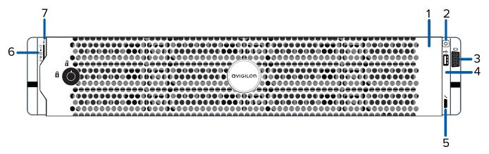
$\textbf{Figure 1:} \ \textbf{Front view of NVR5 Standard 16TB - 64TB recorder with front bezel installed}$
