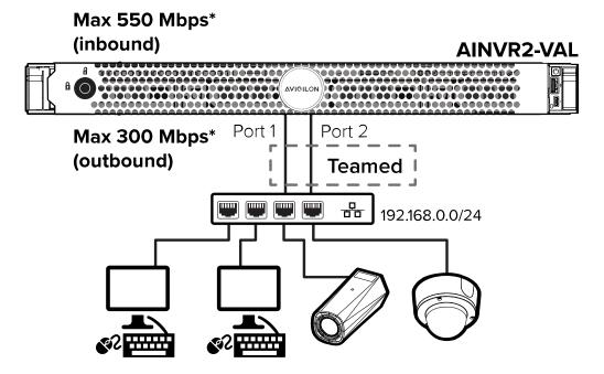
\*The image above shows the inbound and outbound rates of the Al NVR 2 Value 6/12/24 TB. The rates for the Al NVR 2 Value 16 TB are listed in the table under *Network Environment* on page 22.
