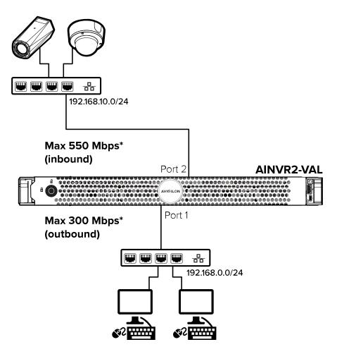
\*The image above shows the inbound and outbound rates of the Al NVR 2 Value 6/12/24 TB. The rates for the Al NVR 2 Value 16 TB are listed in the table under *Network Environment* on page 22.
