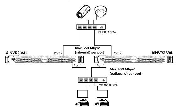
\*The image above shows the inbound and outbound rates of the Al NVR 2 Value 6/12/24 TB. The rates for the Al NVR 2 Value 16 TB are listed in the table under *Network Environment* on page 22.
